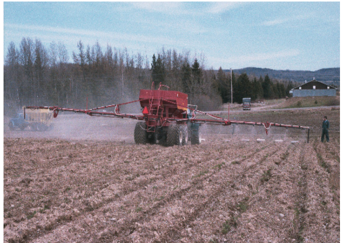
Figure 3. Pneumatic fertilizer spreader operation with collection trays
