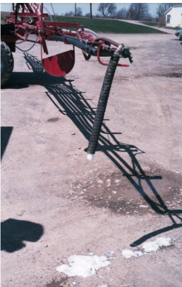
Figure 5. Foam marker system
