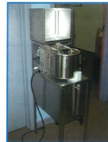
Distillation System Used to Eliminate Minerals, Bacteria and Virtually All Contaminants
