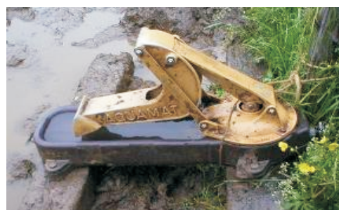
Figure 6. It is preferable to place a pad underneath the nose pump to avoid a mucky drinking area.
