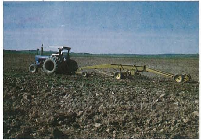
Figure 19. A Land Leveller Implement Performing Land Smoothing.
