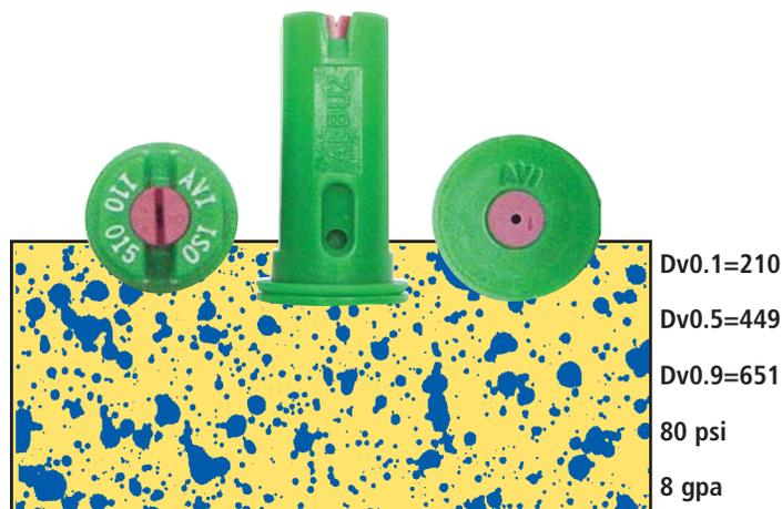
than the metering orifice, causing a significant pressure drop. Even at a gauge pressure of 80 psi, the exit tip pressure may only be 20 to 30 psi. The lower spray pressure at the exit tip causes a narrowing of the fan.
