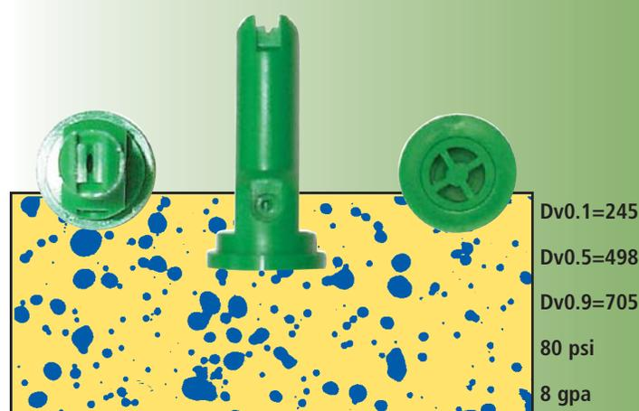
**Hypro AVI, Air-Inducing Venturi.** This nozzle has a two-piece pressure-reducing design that contains a ceramic metering orifice along with a ceramic outer orifice that produces the spray pattern. Ceramic provides for long life and uniform flow rate.
