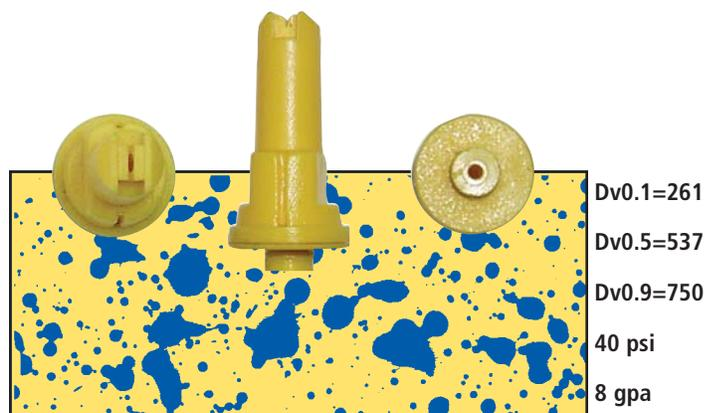
nozzle produces an intermediate spray coarseness droplet as compared to other venturi nozzles, and its optimum pressures are 60 to 80 psi. It has a wider body than a standard nozzle and requires a special nozzle cap. Removal of the insert requires needle-nosed pliers.
