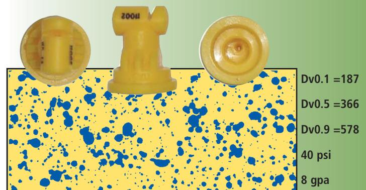
For example, a Turbo TeeJet exit tip can be used to increase spray coarseness, widen the spray angle, and improve pressure operating range. Exit tips must conform to the manufacturer's flow rate recommendations and should be a 110° angle. The TurboDrop nozzle produces droplets of intermediate spray coarseness as compared to other venturi tips. Good patterns are achieved between 30 and 150 psi, while optimum pressures for pesticide effectiveness are 60 to 80 psi.
