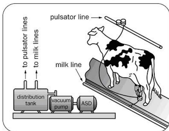
In a vacuum pump upgrade, a farmer changed from two vacuum pumps with a 7.5-hp motor each ([Figure 5](#)) to a vacuum pump with a 10-hp motor and vari-speed control ([Figure 6](#)). This switch resulted in a 5-hp upfront savings and an additional saving on the vari-speed control. The second vacuum pump with a 7.5-hp motor was kept for back-up.
